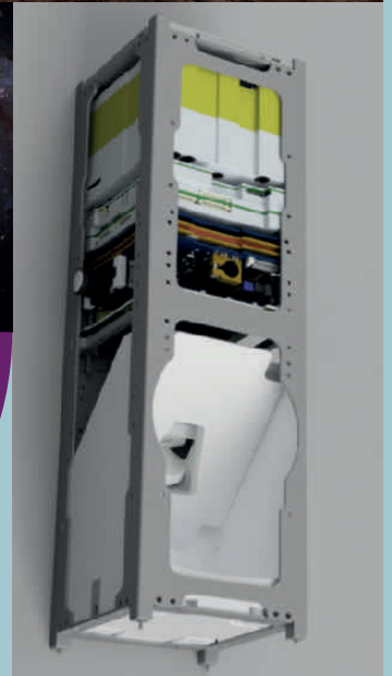
ALIGN Prototype optical communications CubeSat
