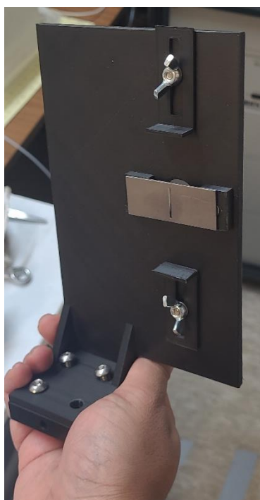
Fig. 1: New capillary holder (left) and a Ni K-edge XANES on 1 wt% Ni /Al 2 O 3 collected through a 0.01 mm thick capillary and an internal diameter of 3 mm.
